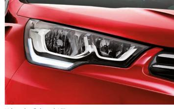
Halogen headlights with LEDs
