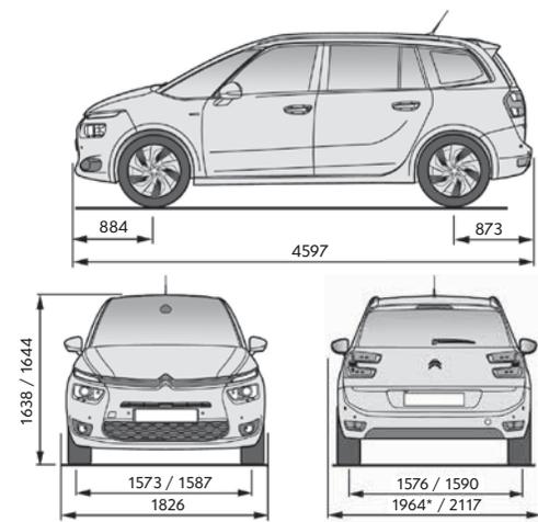
\* Mirrors folded. All measurements are in millimetres.
