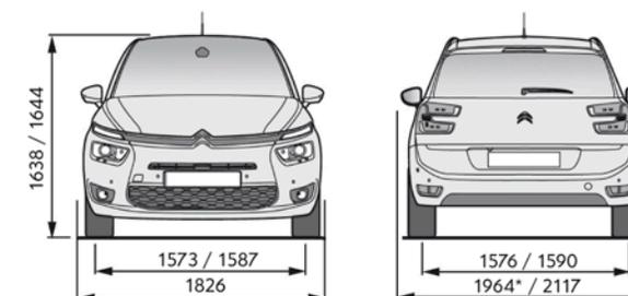
\* Mirrors folded. All measurements are in millimetres.
