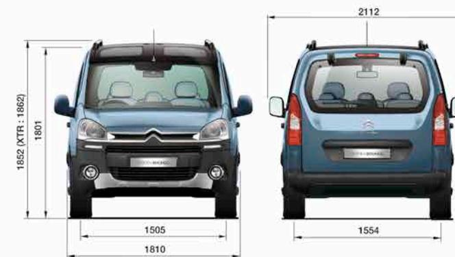
All measurements are in millimetres.
